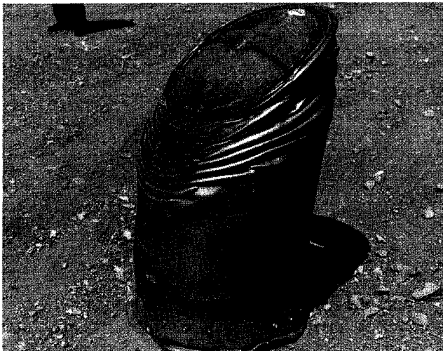
This 500 pound Plutonium Air Transportable (PAT-1) package, shown after impact at 300 mph against an unyielding target, is the type certified by the Commission for air shipment of plutonium. The package consists of a stainless steel containment vessel inside a protective redwood over-pack, all encased within a multi-walled stainless steel drum, as shown in diagram on right.
