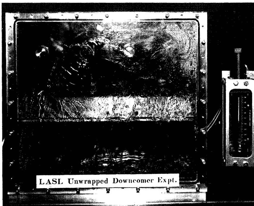
NRC's continuing development of TRAC models is supported by small-scale experiments such as this one shown in progress at LASL. The "unwrapped downcomer" is a 2' x 3' transparent lexon slab which simulates, in a flat configuration, the cylindrical downcomer of a PWR. This device permits researchers to observe two-phase flow (steam-water) phenomena and will enable them to quantify the rates of water entrainment or de-entrainment during a LOCA.
