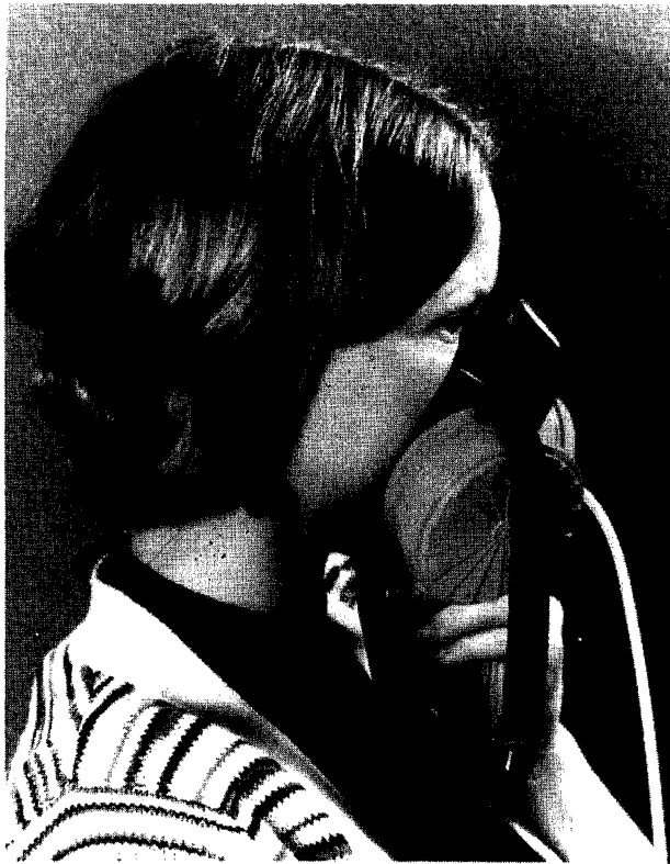
Respirator performance tests conducted at Los Alamos Scientific Laboratory in 1978 are helping NRC develop new guidance on protective equipment used by workers in nuclear facilities. This photo, showing a standard commercial respirator protruding over the user's nose and, thus, failing to "seal" against her smaller-than-average face to offer protection, shows why new guidance is needed.
