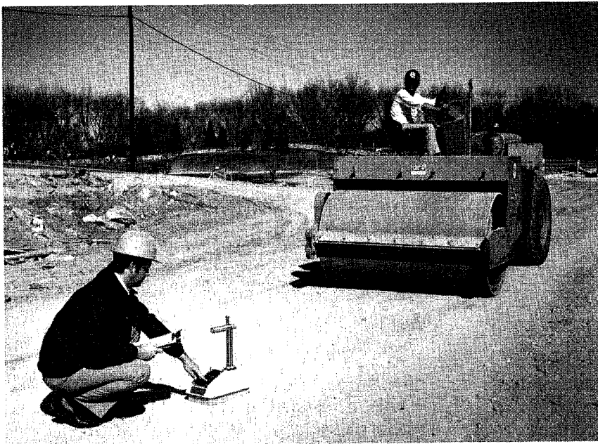
At left, an engineer uses a portable nuclear moisture-density gauge to measure the density (compaction) of a road bed. Below, a workman on the bed of a logging truck uses an extension tool for the removal of a neutron source from the transport shield for placement in a logging tool.
